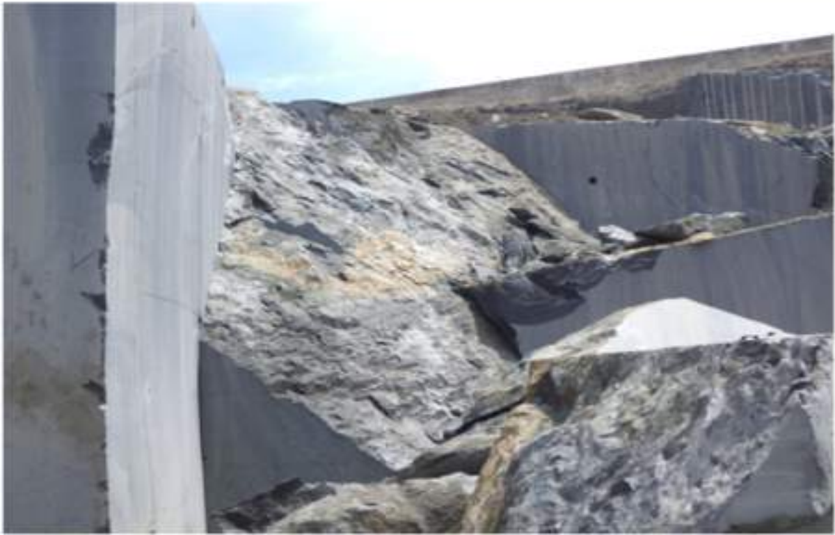
DEFECTIVE SHEAR PLANES WITH NIL PRODUCTION
